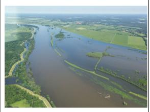
Summary of case study: The main aim of this project was to restore the floodplain habitats, which was brought together with a more comprehensive plan incorporating flood benefits. The dykes containing the River Elbe were to be relocated to allow flooding of the floodplain. An extensive land consolidation process was required. The original dykes were breached but not removed, allowing a dynamic system to evolve over time. Modelling has shown benefits to flood heights both upstream and downstream.
