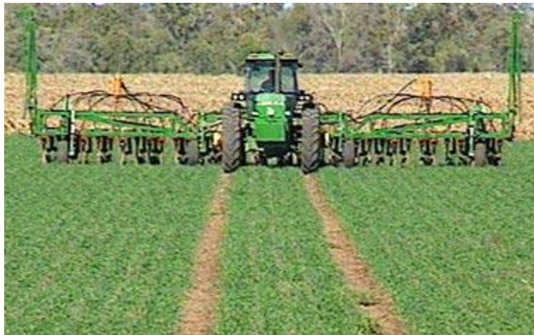
Illustration1: Tractor applying the principle of CTF
